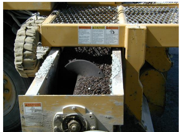
Auger moving chips to the gates.
