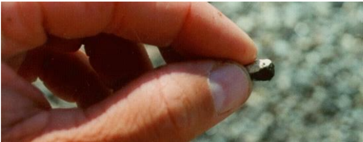
Inspection of aggregate embedment, bituminous material should cover approximately 70%.
