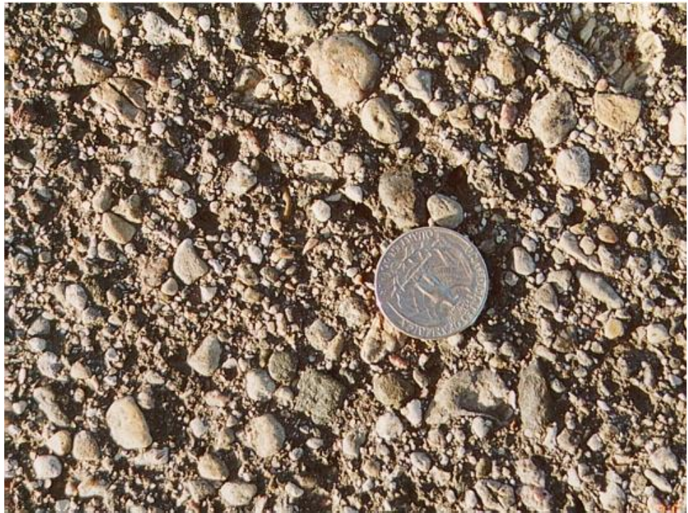
A well graded seal coat aggregate.
