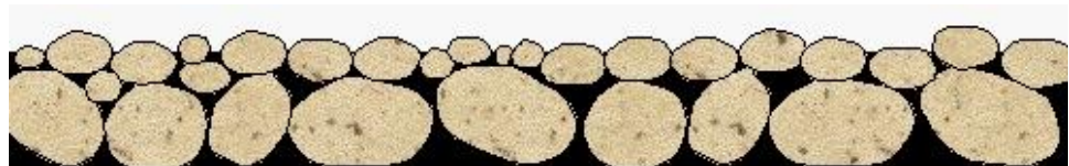
Cross section of a double seal coat.
