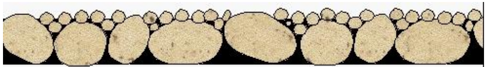
The blotter material will cover up oil, which has bled through.
