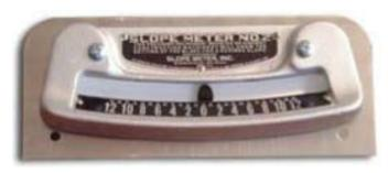
Figure 3. A slope meter accurately displays the percent of cross slope.
