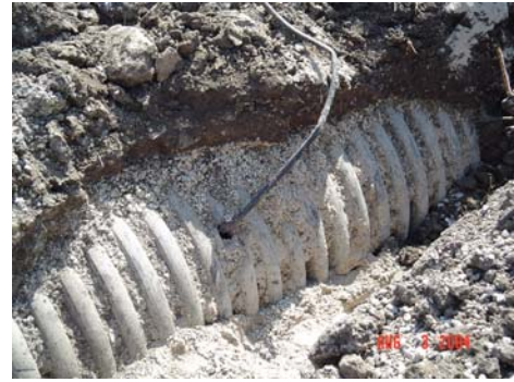
Figure 3. Directional boring damage to plastic culvert.
