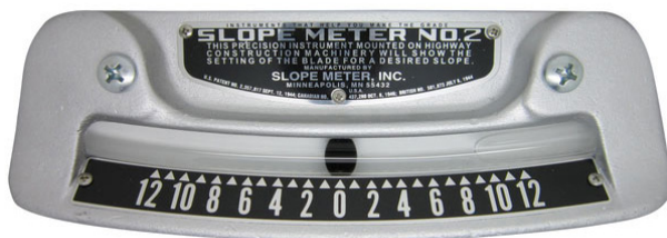
Figure 10-1. Slope meter. Proper cross slope is between 4 and 6. (Source: tigersupplies.com)
