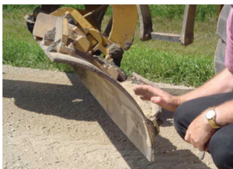
Figure 8-2. Tilt the blade forward for dragging. (Source: FHWA Gravel Roads Construction & Maintenance Guide)
