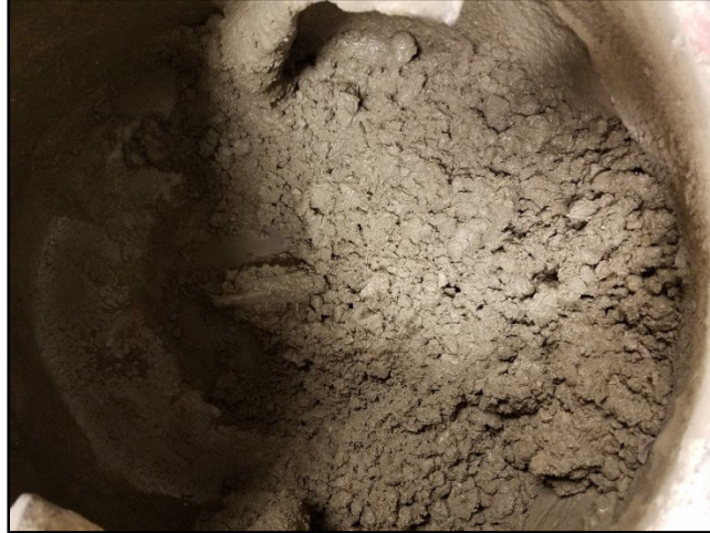
Figure 22. Photo of Mix B4 in the mixer with 15 mL HRWR (15.2 fl oz/yd 3 ).
