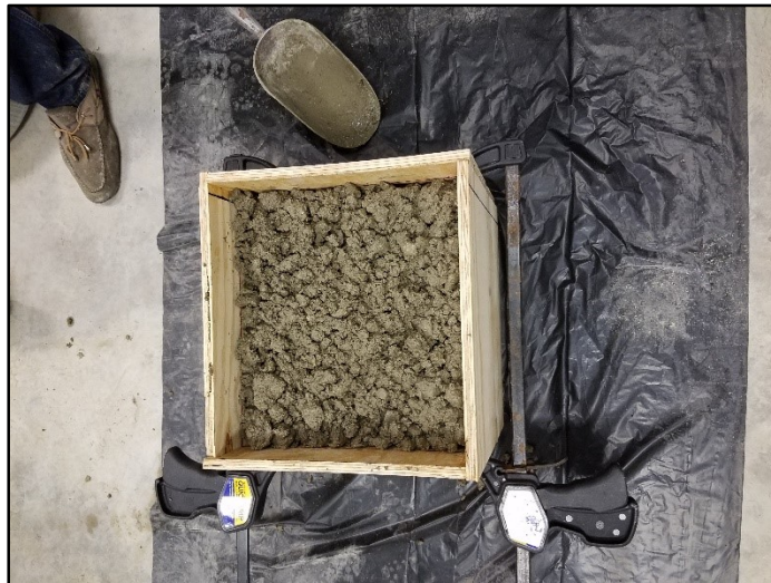
Figure 23. The box is filled prior to vibration.
