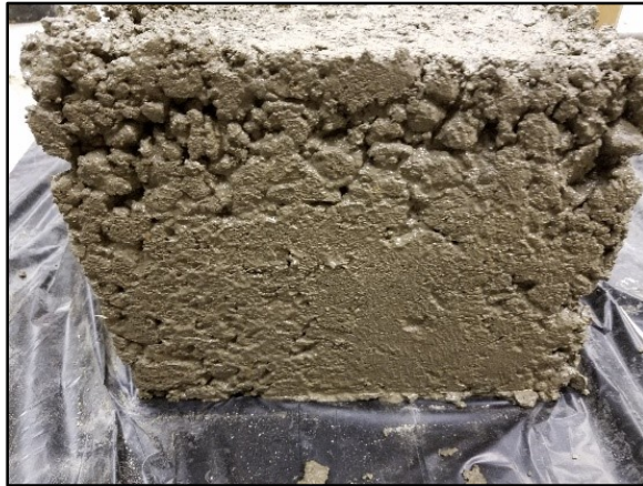
Figure 28. 60.9 fl oz/yd 3 : Bottom portion is fairly well consolidated – optimum dosage.
