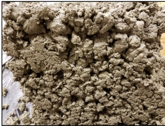
Figure 25. The surface voids are evaluated. This is obviously not adequate at this stage.
